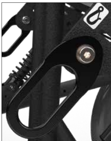
Attachment points, front according to ISO 7176-19
