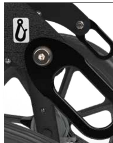
Attachment points, rear according to ISO 7176-19
